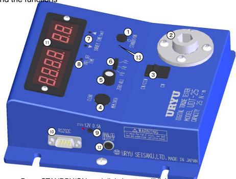
①Power switch: Press STANDBY/ON, and digital meter will light.
