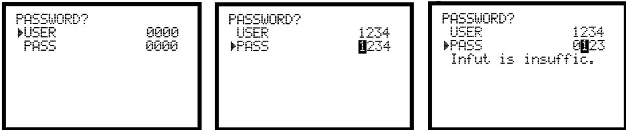
Press **ENT** after you arranged numbers for USER and PASS as necessary. Then press **RES** to get out of setup MODE, and the registration will be completed. These passwords of USER and PASS will be operative from next operation. UCC will detect insufficient number as an error if you enter different number.
