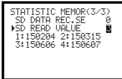
Enter left figure of file name, and UCC will download setup value stored in SD card. Above picture (right) shows entry of 3 downloading file 150606. Fix digit number like [SD(6 digit only)] when you name file by PC. UCC will not display setup value if digit number is less than 6.
