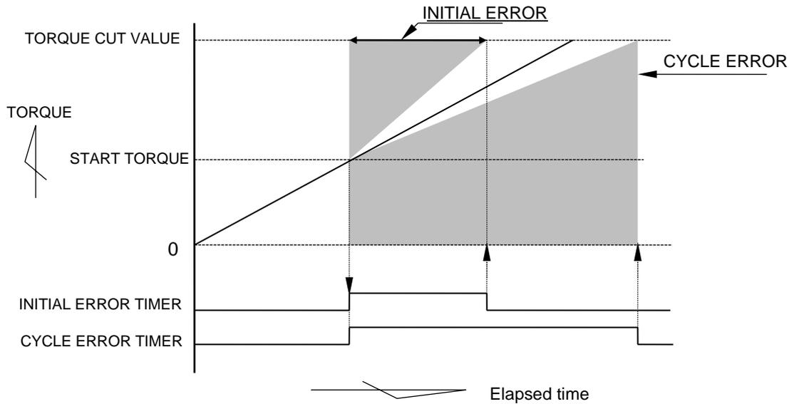
Note) This line graph describes torque-time relations when torque grows rectilinearly.
