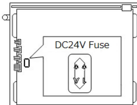
Use URYU genuine fuse whose code number is 909-814-0 Fuse HM10(1A). When replacing fuse Damaged by short-circuit, fix the short-circuit problem first. Fuse replacement without fixing the problem repeat the same trouble.
