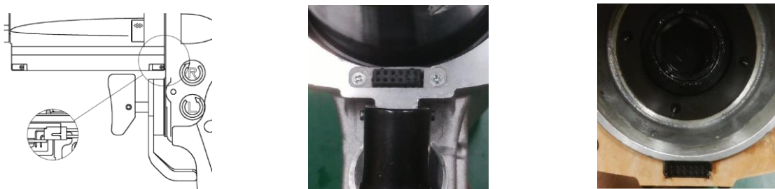
Enlarged Pictures of Connector between Handle and Front Casing
